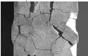
10 Disruptive action of 10% sodium sulphate solution on mortar sample colour print on inside back cover
