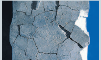
10 Disruptive action of 10% sodium sulphate solution on mortar sample (page 13)
