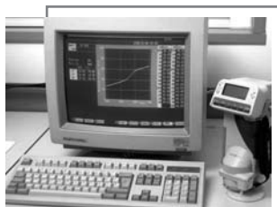
Colour measurement using a portable colorimeter; the results are plotted on a computer screen
