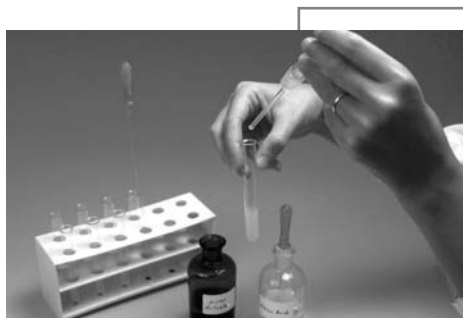
15 Microchemical test for chloride identification.
