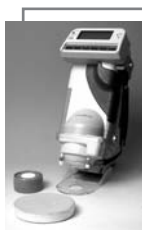
A portable colorimeter and test sample colour print on inside back cover
