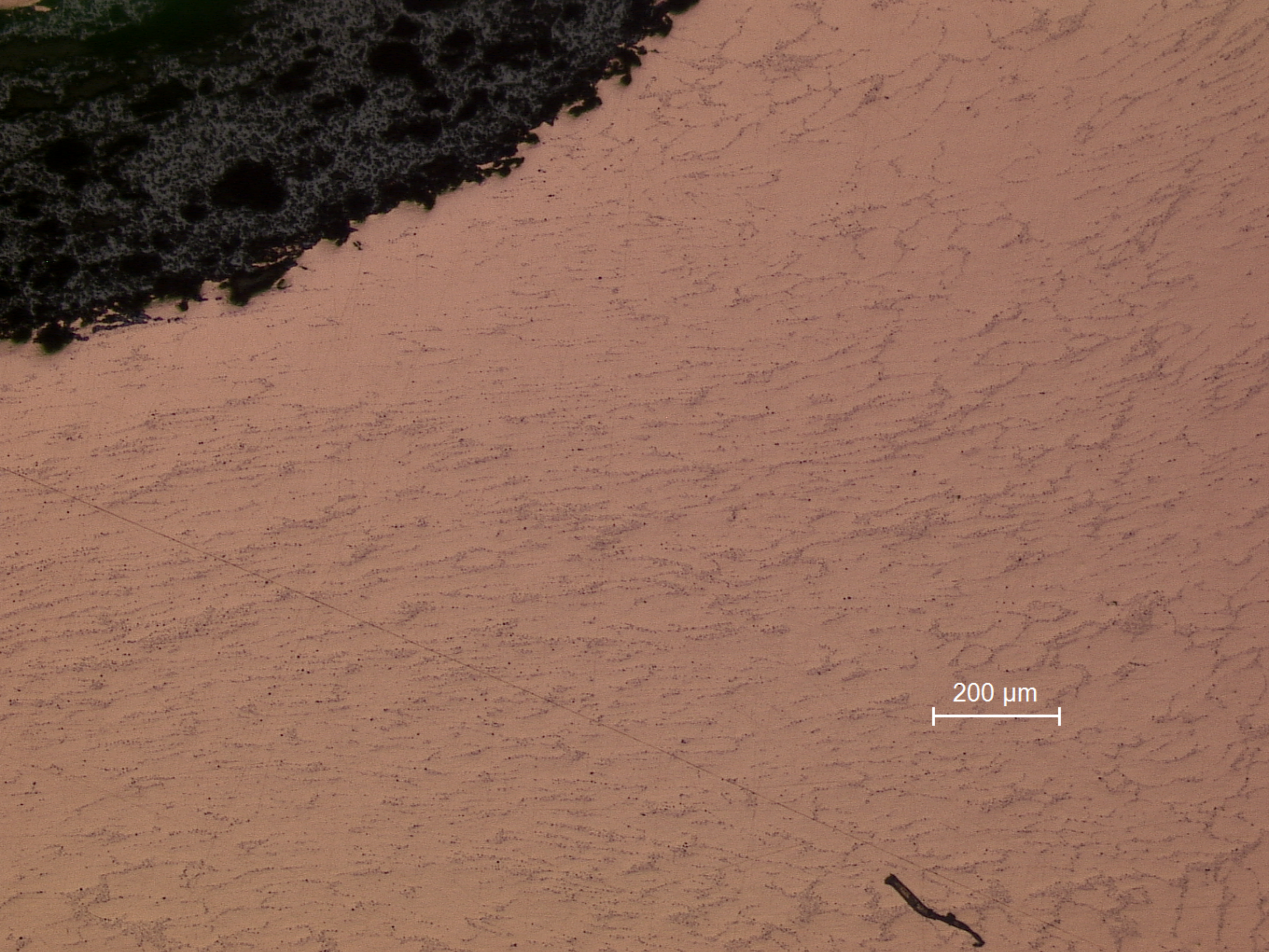
B44.1 General view: the net of small inclusions delineates the grains, which are elongated following the direction of working.
