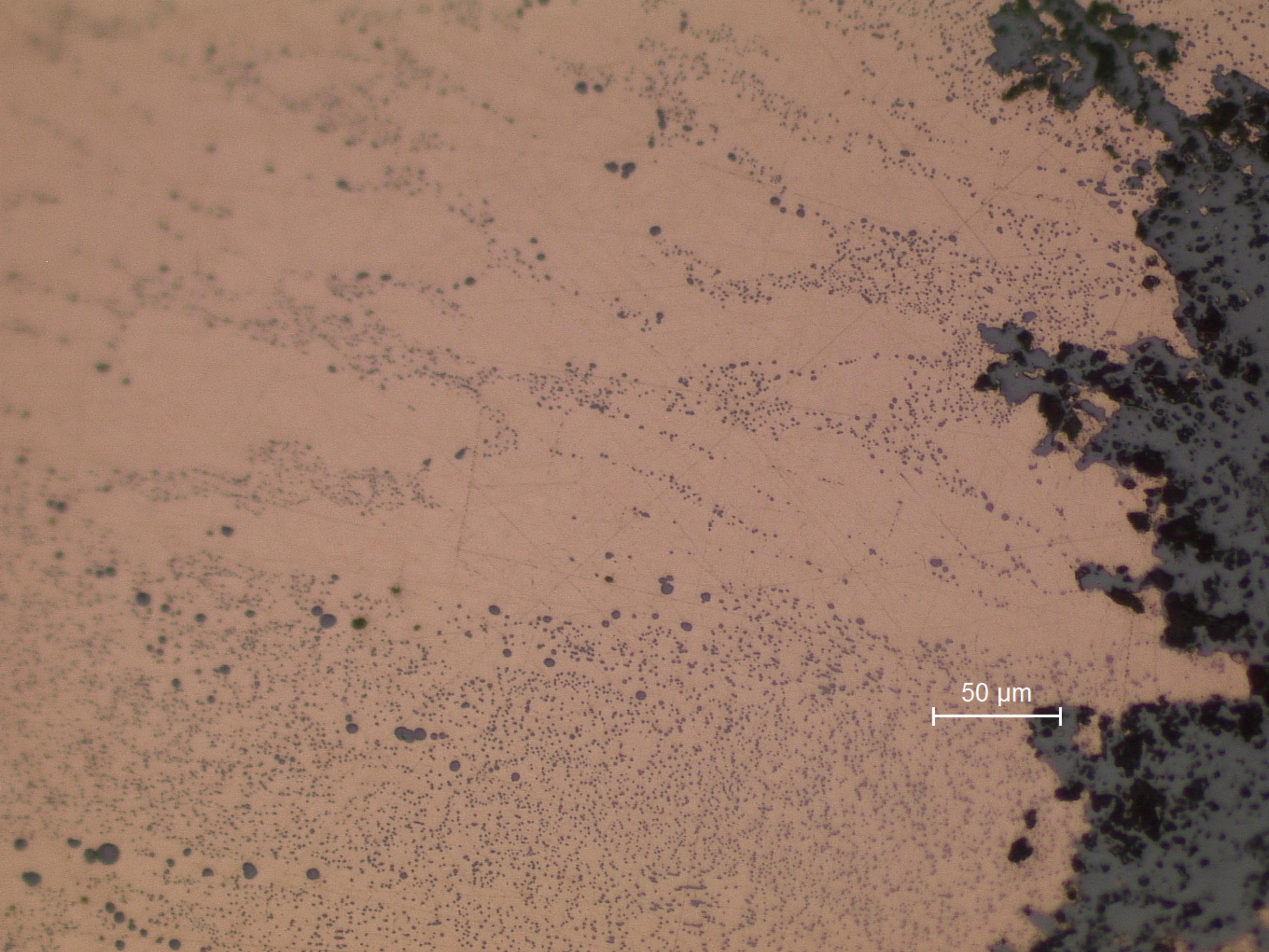
B44.6 Detail showing the preferential situation of the globular inclusions along the grain boundaries.
