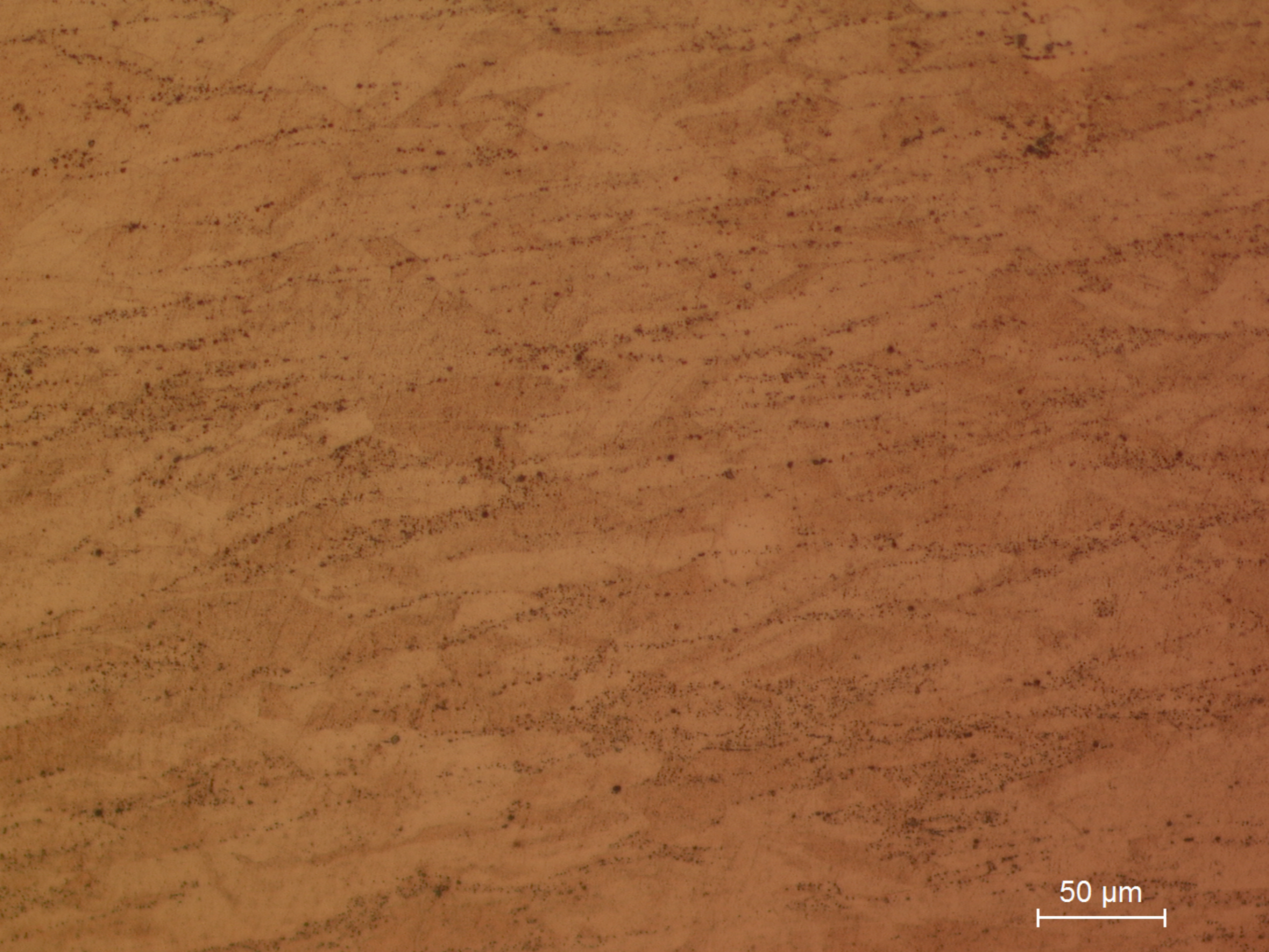
B44.4 Detail showing the elongation of the grains (etchant: aqueous \text{FeCl}_3 ).
