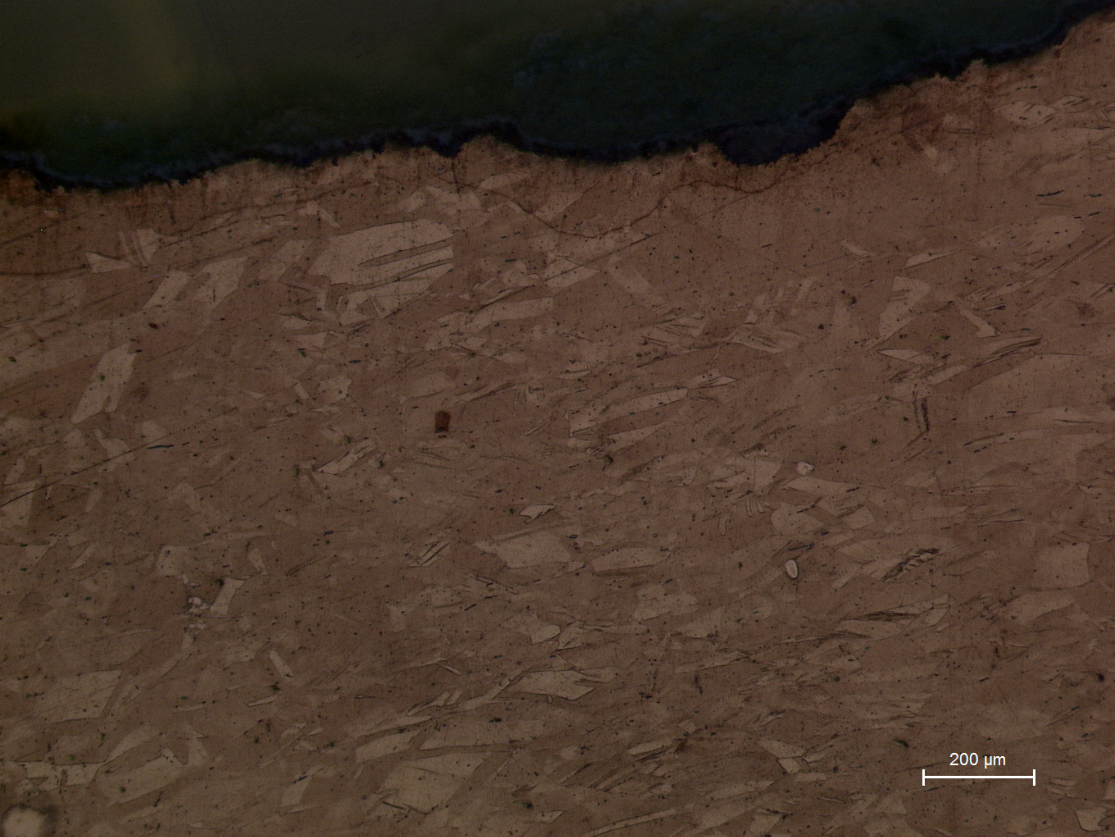
B09.1 General view showing polygonal grains which are deformed in the direction perpendicular to striking; presence of annealing twins and some strain lines (etchant: aqueous \text{FeCl}_3 ).
